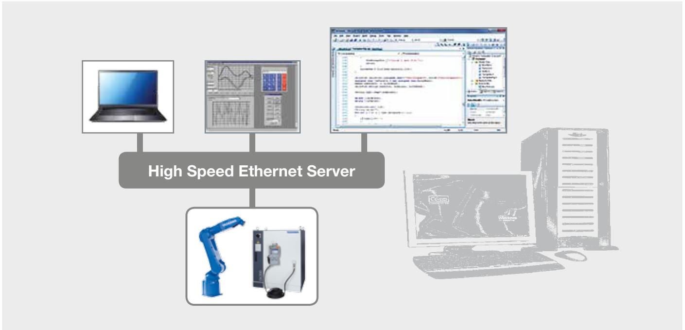
The High Speed Ethernet Server protocol is the current “General purpose” protocol for communication between the DX200 and external devices. It provides a higher performance and functionality over the older protocols like EServer thus it’s the recommended protocol for developing new applications.
