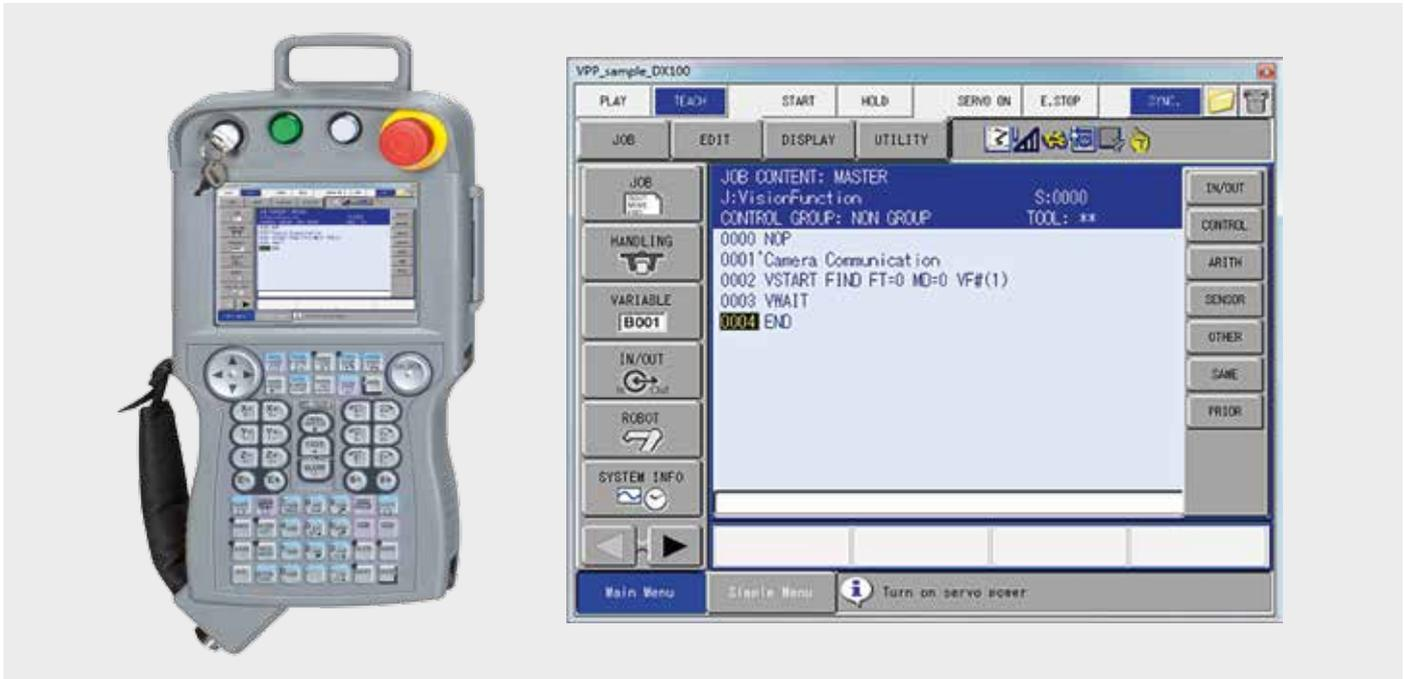
This function is an inform instruction to communicate with different Vision System. It maps the communication protocols of a variety of selected vision systems and works, dependent on these, on the basis of Ethernet or RS232. This robot instruction allows easy control of image processing devices.
