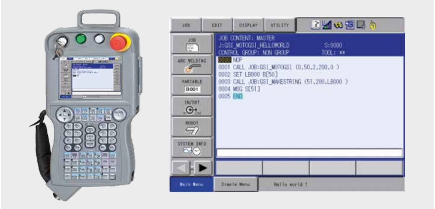
MotoGSI is a development package for creating communication interfaces on job basis. It comes with a set of jobs which allow communication with nearly every external device that supports Ethernet/TCP, Ethernet/UDP or RS232-connections. It also provides a set of helper functions to process and convert the in- and outgoing datastreams which are based on byte arrays. Also included in the package is a set of sample jobs to demonstrate the way of programming.
