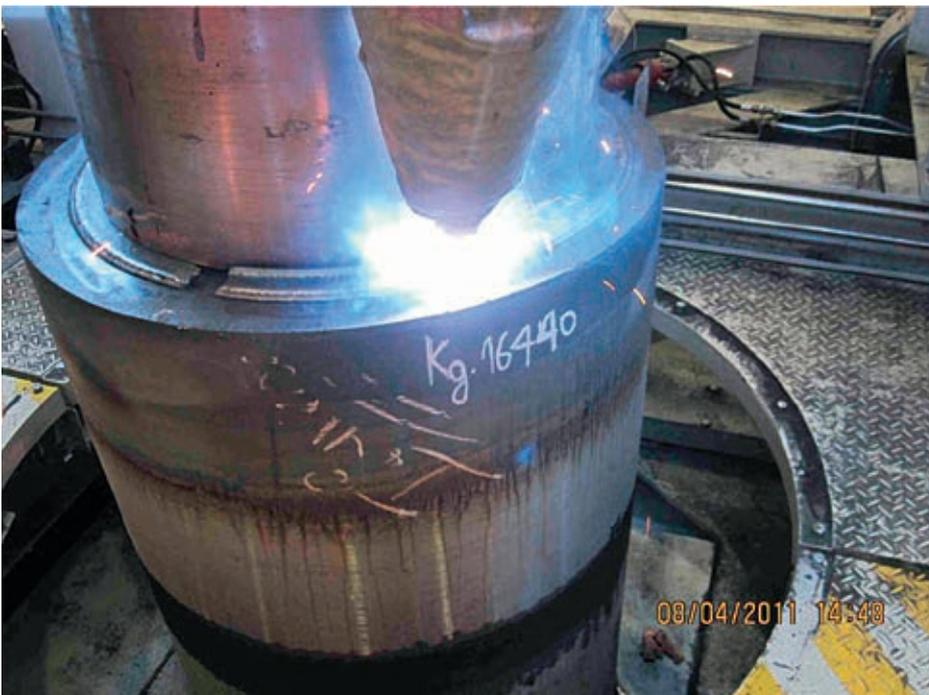
Example for multi layer welding on electrodes for ESR process:
