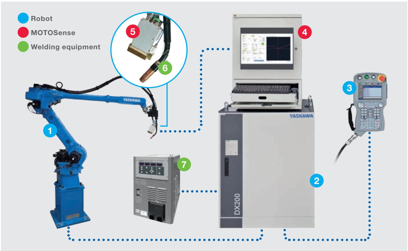
**Components of adaptive robotic welding cell:**
