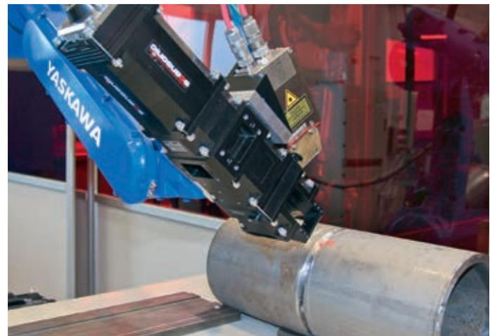
Seamtracking with laserwelding unit
