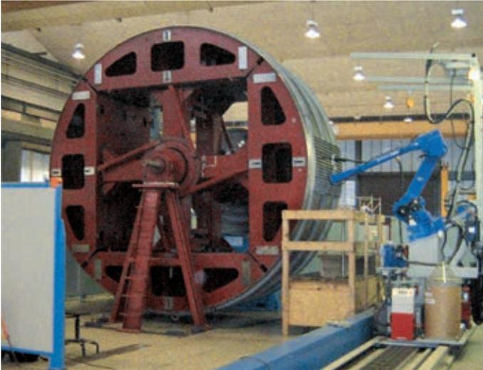
*System for the welding of machine components for the paper industry*
