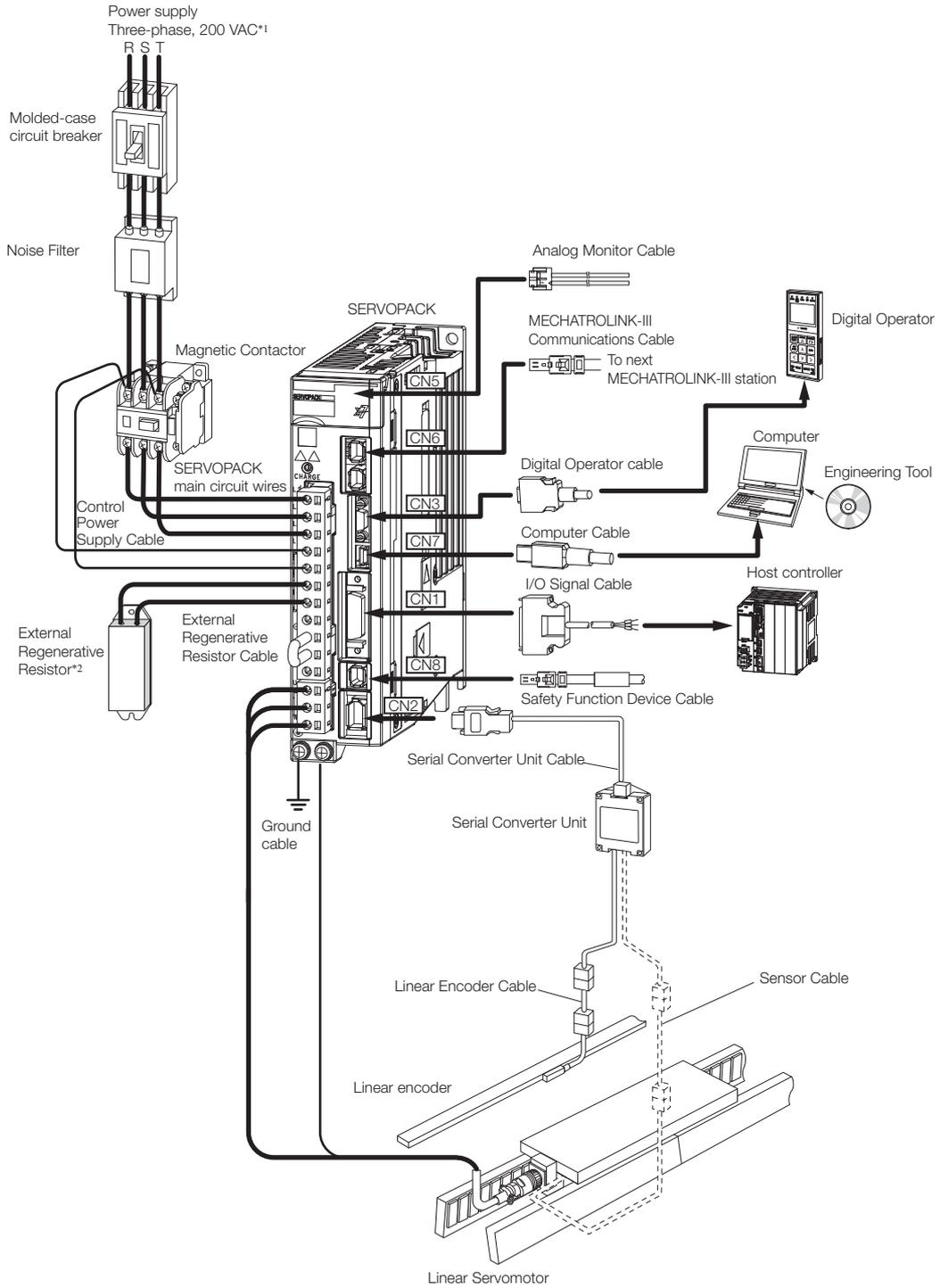
\*1. This example is for a SERVOPACK with a three-phase, 200-VAC power supply input. The pin layout of the main circuit connector depends on the voltage.
