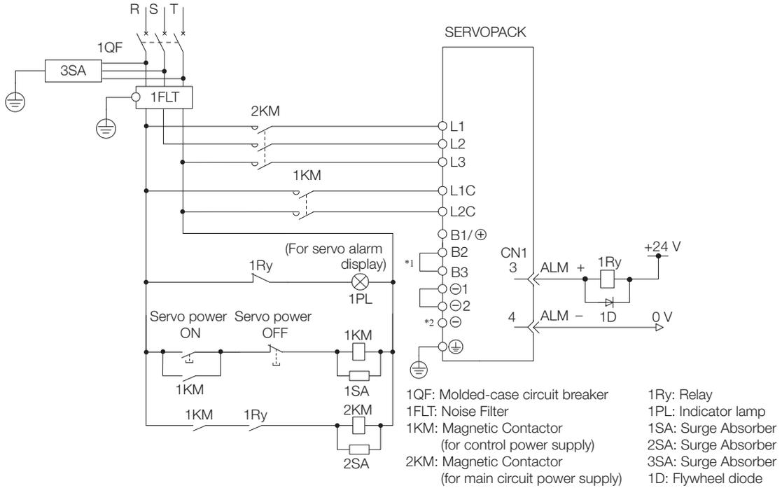
\*1. You do not have to connect B2 and B3 for the following models: SGD7S-R70A, SGD7S-R90A, SGD7S-1R6A, and SGD7S-2R8A. Do not connect them.
