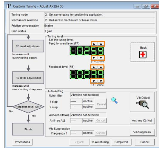
**Information** The new feedforward level will not be used until the positioning completed signal is output.
