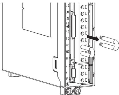
2. Connect the External Regenerative Resistor between the B1/⊕ and B2 terminals.
