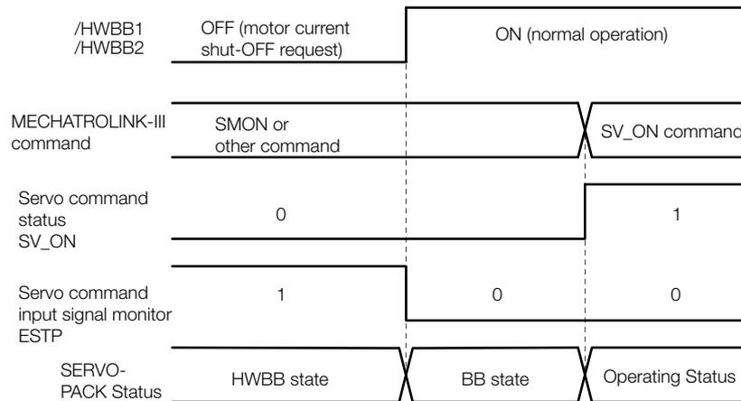
If the /HWBB1 and /HWBB2 signals are OFF and the SV\_ON (Servo ON: 31h) command is received, the HWBB state will be maintained even after the /HWBB1 and /HWBB2 signals are turned ON. Send the SV\_OFF (Servo OFF: 32h) command to place the SERVOPACK in the BB state and then send the SV\_ON (Servo ON: 31h) command.
