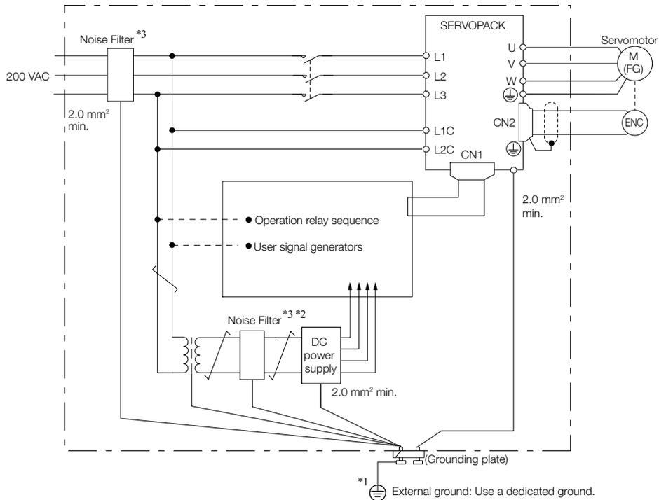
\*1. For the ground wire, use a wire with a thickness of at least 2.0 mm<sup>2</sup> (preferably, flat braided copper wire).
