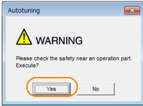
The Servomotor will start operating and tuning will be executed. Vibration that occurs during tuning will be detected automatically and suitable settings will be made for that vibration. When the settings have been completed, the indicators for the functions that were used will light at the lower left of the dialog box.
