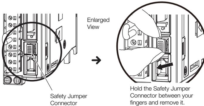
2. Connect the safety function device to the connector for the safety function device (CN8).
