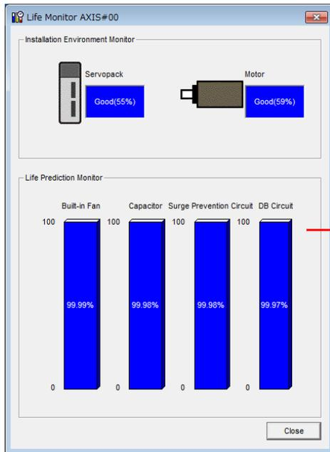
A value of 100% indicates that the SERVOPACK has not yet been used. The percentage decreases as the SERVOPACK is used and reaches 0% when it is time to replace the SERVOPACK.
