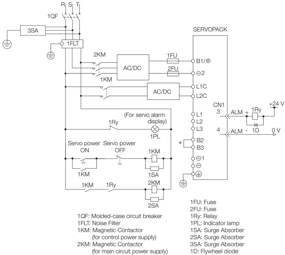
\* You do not have to connect B2 and B3 for the following models: SGD7S-R70A, SGD7S-R90A, SGD7S-1R6A, and SGD7S-2R8A. Do not connect them.
