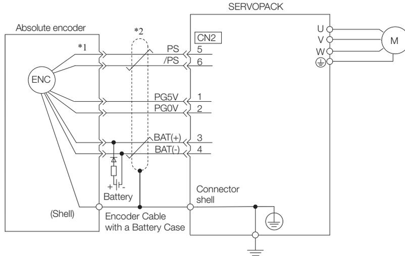
\*1. The absolute encoder pin numbers for wiring the connector depend on the Servomotor that you use.
