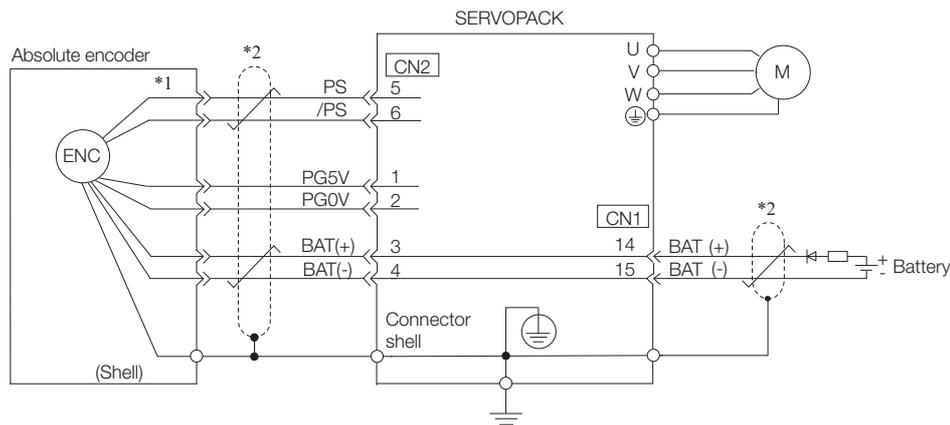
\*1. The absolute encoder pin numbers for wiring the connector depend on the Servomotor that you use.
