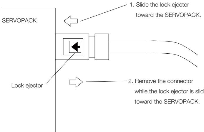
Note: The MECHATROLINK-III Communications Cable connector may be damaged if it is removed without being unlocked.
