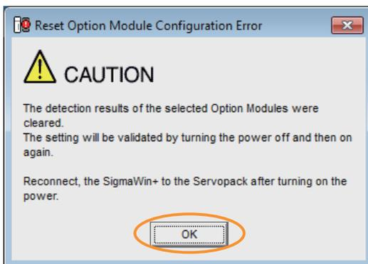
7. Turn the power supply to the **SERVOPACK OFF** and **ON** again.
