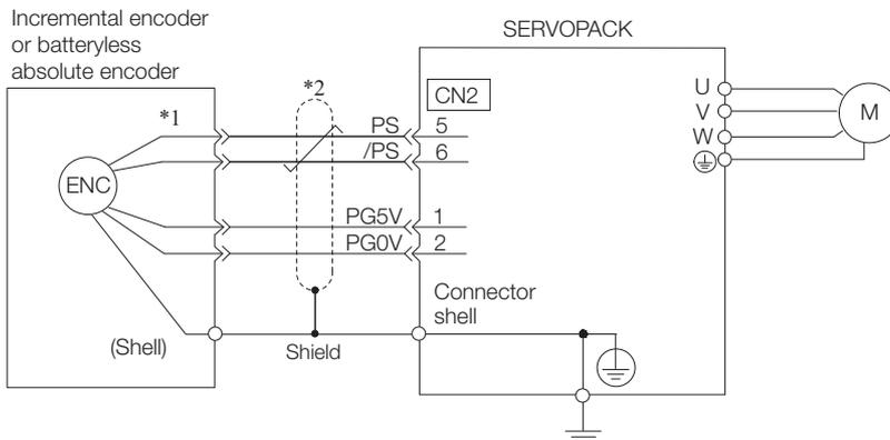
\*1. The encoder pin numbers for wiring the connector depend on the Servomotor that you use.
