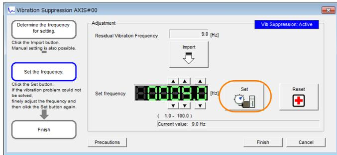
If the vibration is not eliminated, use the ▲ and ▼ Buttons for the set frequency to fine-tune the value and click the **Set Button** again.
