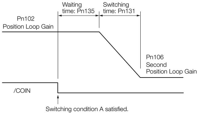
**Information** You can use gain switching for either PI control or I-P control (Pn10B = n.□□□□ or □□1□).
