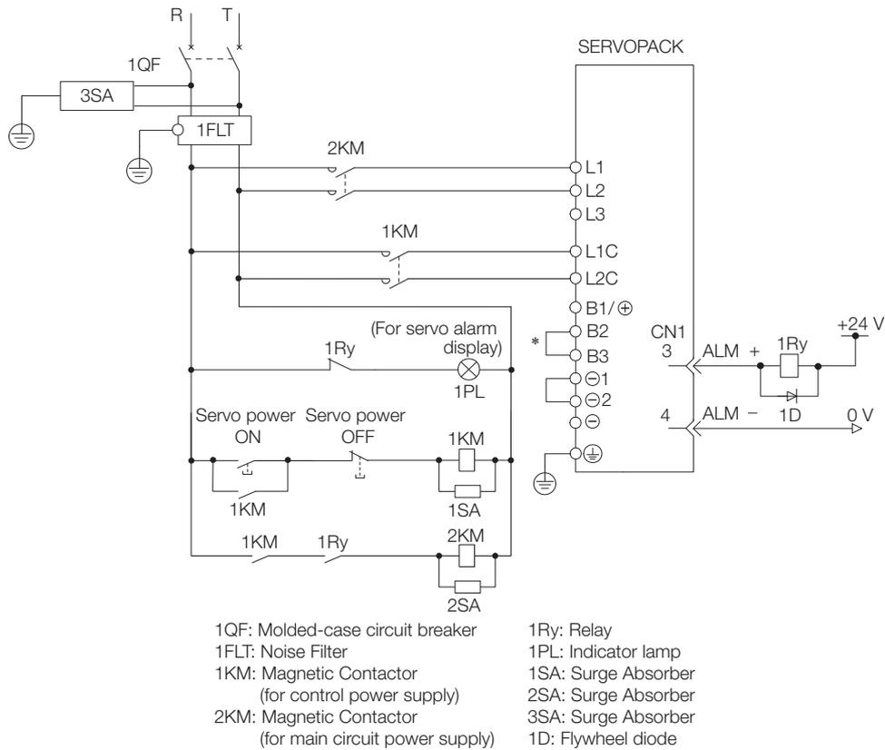
\* You do not have to connect B2 and B3 for the following models: SGD7S-R70A, SGD7S-R90A, SGD7S-1R6A, and SGD7S-2R8A. Do not connect them.
