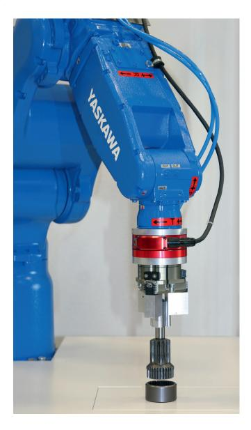
MotoFit alters the robot's position based on the force encountered to align or assemble parts. (During normal robot operation, the robot is setup for positional control. It moves to or retains position even when external forces are applied, provided that forces do not exceed limits that would cause an error.)
