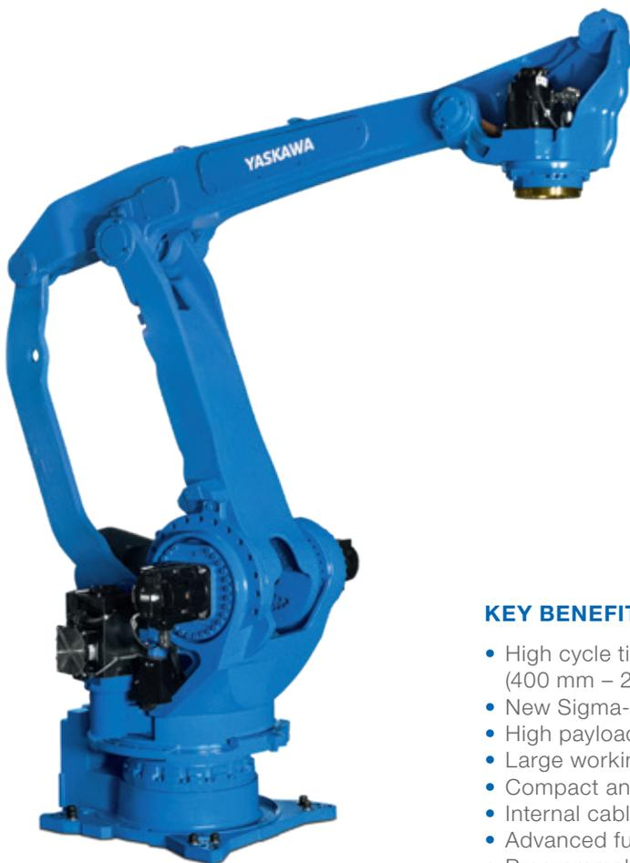
The fast 4-axis MOTOMAN PL190-100 achieves top performance with over 2000 cycles per hour for box, carton and pack palletizing in final packaging and logistics.
