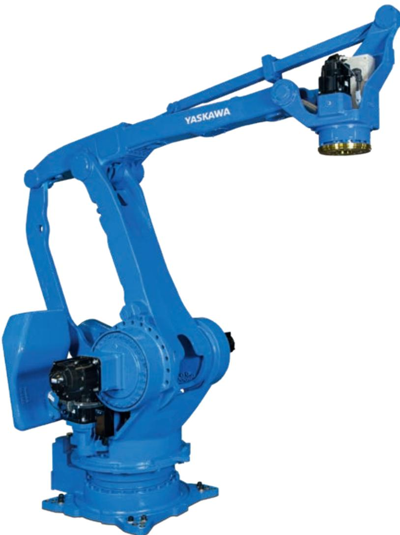
The most powerful 4-axis robot of the PL-series is the MOTOMAN PL800 with a payload of 800 kg. This palletizer offers high performance for box, carton and pack palletizing in versatile end-of-line packaging and logistics applications. The large working range with a maximum reach of 3159 mm and an achievable stacking height of over 2624 mm allows versatile use across all palletizing applications.
