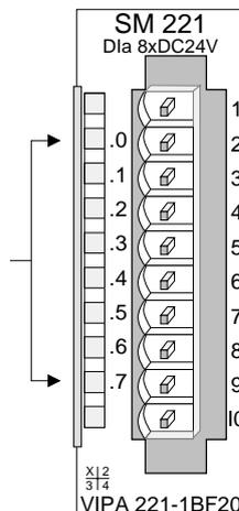
**Wiring and schematic diagram**
