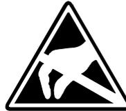
The symbol is located on the module, the module rack or on packing material and it indicates the presence of electrostatic sensitive equipment.
