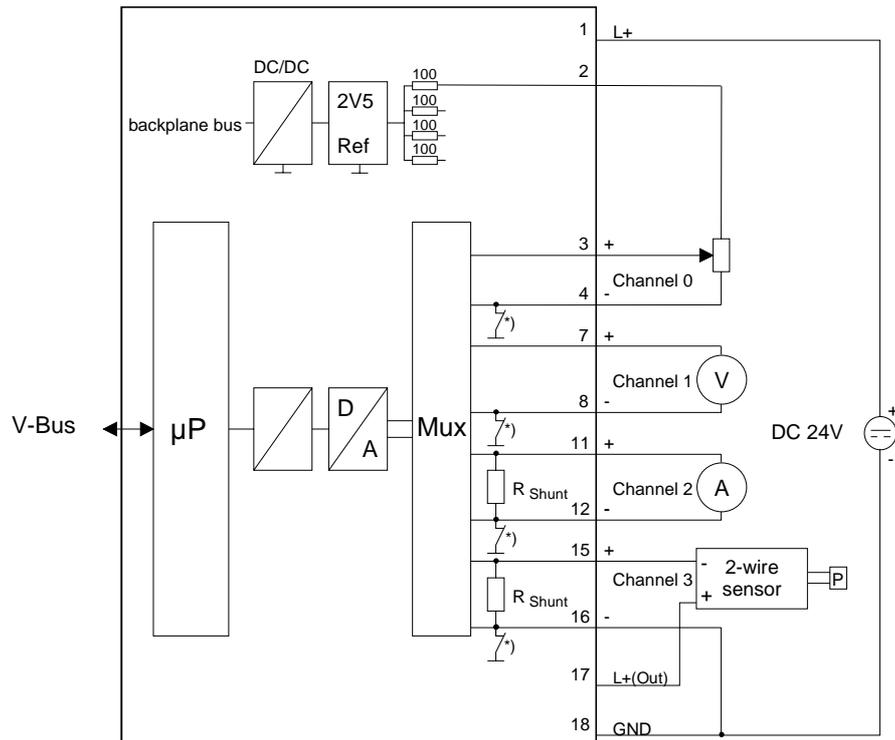
\*) During measuring the connection to ground is closed.
