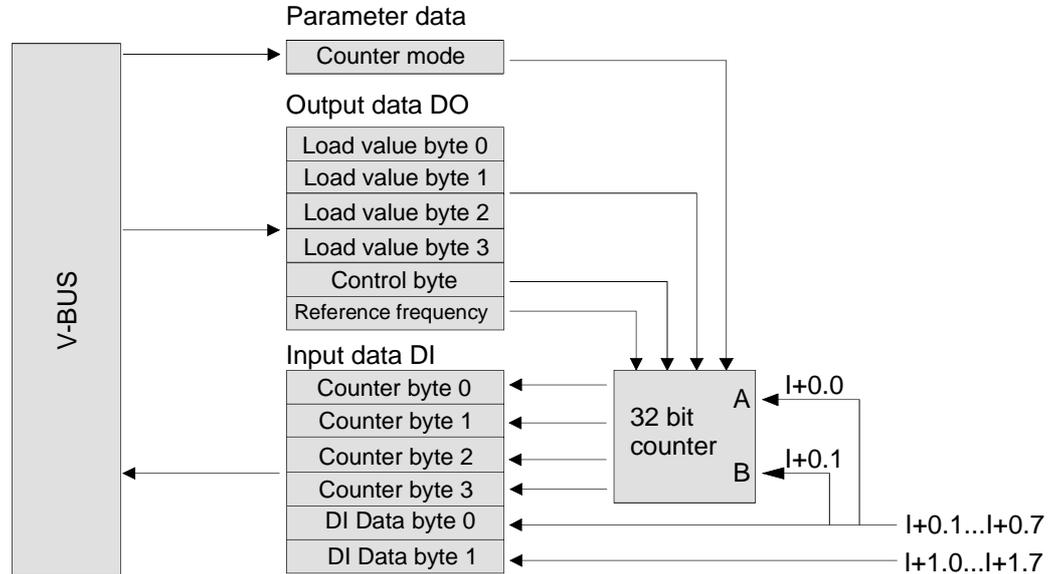
By writing *output data DO* to the module, you may preset a counter value with a *load value* as well as a *reference frequency*. The activation of this values takes place by means of the *control byte*.
