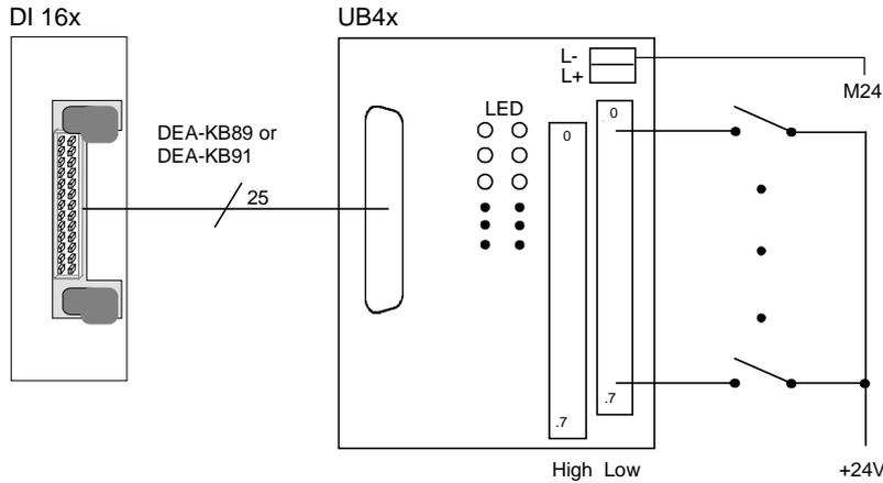
Schematic diagram module
