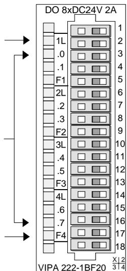
**Wiring and schematic diagram**
