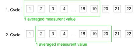
Analog part > Analog part - Parameterization
