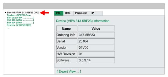
Here order number, serial number and the version of firmware and hardware of the CPU are listed. [Expert View] takes you to the advanced "Expert View".
