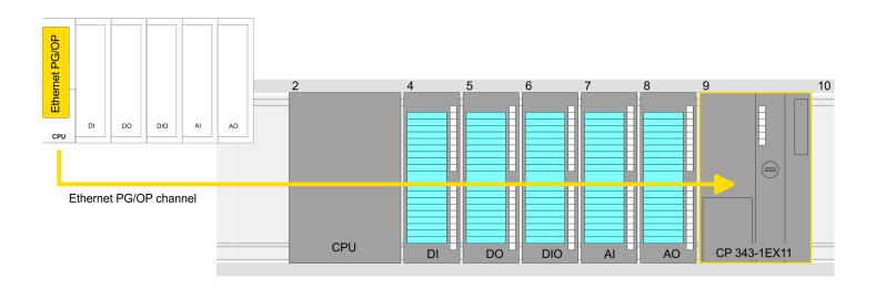
TIA Portal - Hardware configuration - Ethernet PG/OP channel
