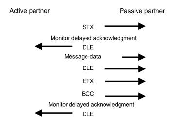
When a DLE is transferred as part of the information it is repeated to distinguish between data characters and DLE control characters that are used to establish and to terminate the connection (DLE duplication). The DLE duplication is reversed in the receiving station.
