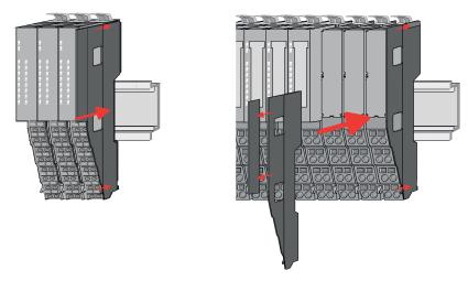
7. After mounting the whole system, to protect the backplane bus connectors at the last module you have to mount the bus cover, now. If the last module is a clamp module, for adaptation the upper part of the bus cover is to be removed.
