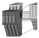
**6.** To mount the module put it to the gap between the both modules and push it, guided by the stripes at both sides, to the mounting rail.
