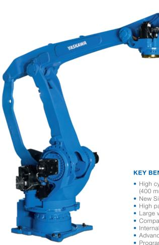
With over 1400 cycles per hour, the fast and powerful 4-axis MOTOMAN PL320 robot offers top performance for box, carton and bag palletizing for end-of-line packaging and logistics applications.
