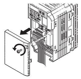
Figure 4 Remove the Front Cover
