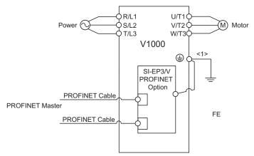
Figure 20 Wiring Diagram
