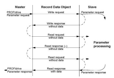
Figure 23 PROFIdrive Acyclic Parameter Access Mechanism Structure
