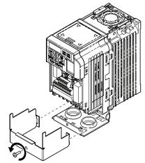
Figure 8 Remove the NEMA Type 1 Terminal Cover
