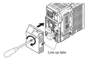
Figure 21 Attach the Option Cover
