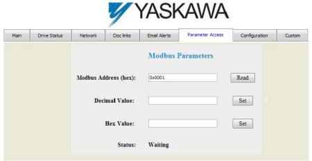
Figure 29 Parameter Access Tab View
