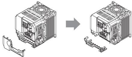
Figure 6 Remove the Terminal Cover and Bottom Cover on an IP20/Open-Chassis Drive (Models CIMR-V□□BA0006B to BA0018B; 2A0010B to 2A0069B; 4A0001B to 4A0038B)
