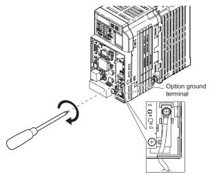
Figure 17 Connect the Ground Wire to the Option
