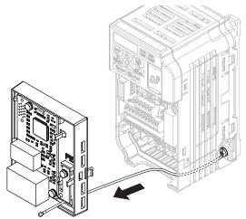
Figure 15 Ground Wire Routing
