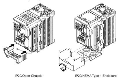
Figure 12 Reattach the Bottom Cover
