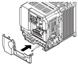
Figure 13 Reattach the Terminal Cover (Models CIMR-V□BA0006□ to BA0018□; 2A0010□ to 2A0069□; 4A0001□ to 4A0038□)
